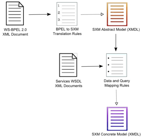
Fig. 1. The translation architecture of BPEL processes to abstract and concrete SXM models.
