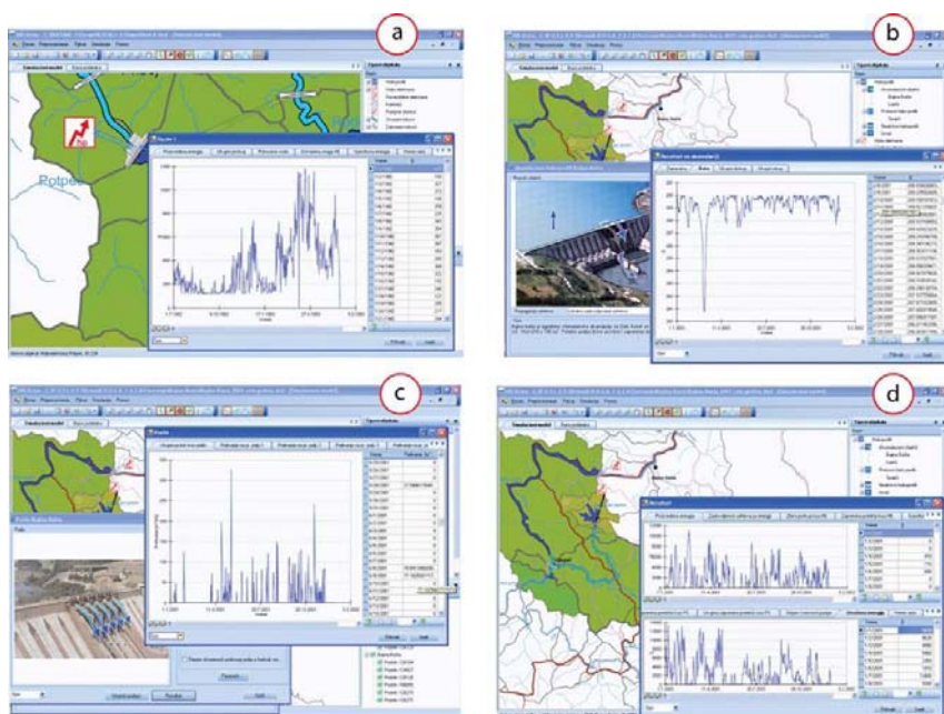
Figure 4 Simulation outputs (a - Potpeć HPP power generation, b - Water level of the Kokin Brod Reservoir).
