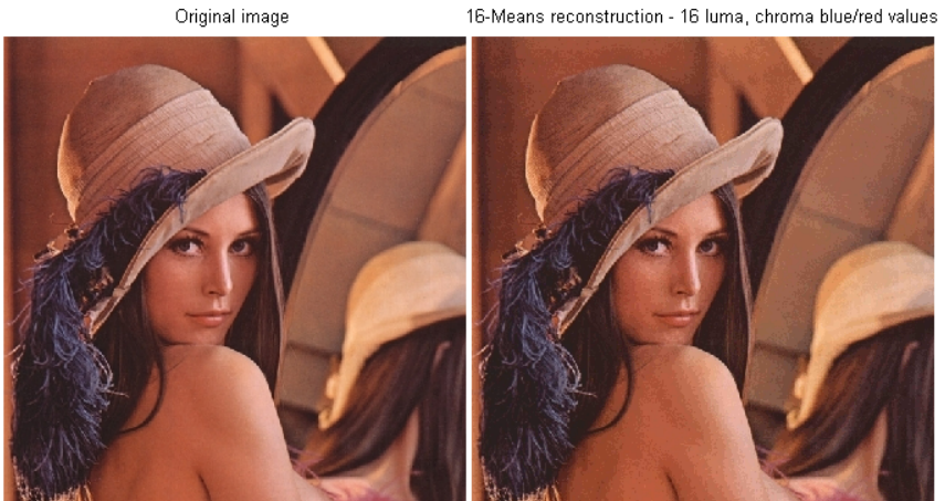
Figure 5 Fast 16-Means Luma-Chroma Quantization of Lena image (16 luma levels, 16 chroma blue/red levels).
